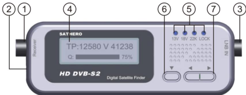
1. Receiver connecting port and power supply connection.
